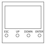
The main menu is accessed by pressing the Mode/Esc-button, Browse through the submenu by pressing Up or Down .Press the Enter-button in order to select the desired menu. You can change the selection by pressing Up or Down, confirm every selection by pressing the Enter-button. You can leave every mode by pressing the Mode/Esc-button. The functions provided are described in the following setting.
