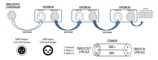
For installations where the DMX cable has to run for a long distance, or as an electrically noisy environment, it is recommended to use a DMX terminator. This helps in preventing corruption of the digital control signal by electrical noise. The DMX terminator is simply an XLR plug with a 120 resistor connected between pins two and three, which is then plugged into the output XLR socket of the last fixture in the chain.
