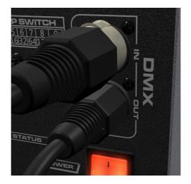
*Address Setup* – Use the DIP switch located on the rear of the machine to set the DMX address. The machine occupies 2 control channels. The starting address is defined as the first channel from which the machine will respond to the controller. Always double check to make sure there are no overlapping channels in order to control the machine correctly.
